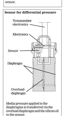
ETP90 is directly connected to the media without the need for pressure intermedia. This eliminates the problems usually associated with pressure intermedia, such as temperature drift. Since ETP90 does not use pressure intermedia temperature influence is very low. ETP90 is both temperature- and longterm stable.
